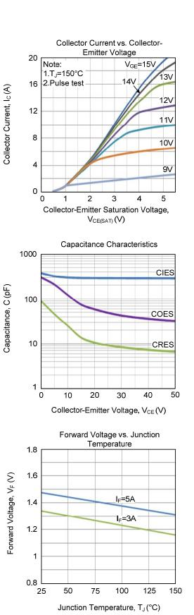
Insulated Gate Bipolar Transistor
