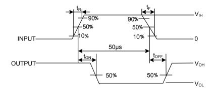
Notes: 1. Pulse width 50 $\mu$ s, duty cycle 10%, Output impedance 50 $\Omega$ ,  $t_R \le 5$ ns,  $t_F \le 10$ ns.
