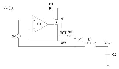
If both  $V_{IN}$  and EN are higher than their appropriate thresholds, the chip starts. The reference block starts first, generating stable reference voltage and currents, and then the internal regulator is enabled. The regulator provides stable supply for the remaining circuitries.
