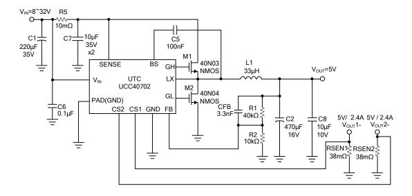
$\begin{aligned} &V_{OUT}\text{=}V_{FB}\times(1\text{+}R1/R2),\,V_{FB}\text{=}1.00V,\,R2\text{ suggest }1\text{k}^{\sim}30\text{K}\Omega\\ &I_{SEN}\text{=}2.63\text{A}\left(I_{SEN}\text{=}V_{CS}(0.1\text{V})\,/\,\text{RSEN}(38\text{m}\Omega)\right) \end{aligned}$
