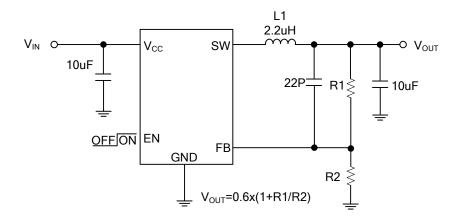
$V_{OUT}=V_{FB} \times (1+R1/R2)$ ,  $V_{FB}=0.6V$ , R2 suggest  $60k^{\sim}300k\Omega$
