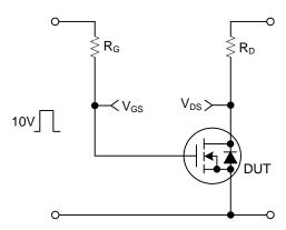
Resistive Switching Test Circuit
