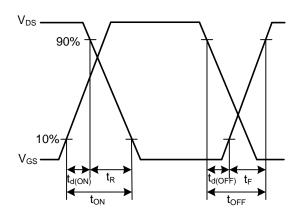
Resistive Switching Waveforms
