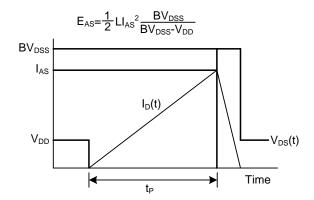
Unclamped Inductive Switching Waveforms
