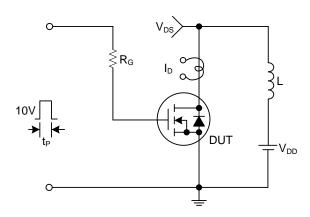
**Unclamped Inductive Switching Test Circuit**
