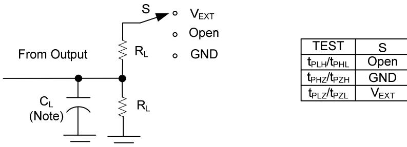
Note:  $C_L$  includes probe and jig capacitance.
